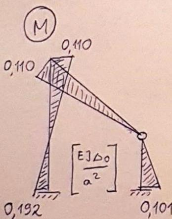
PRZEMIĘSCZENIE PUNKTU B / POINT B DISPLACEMENT
